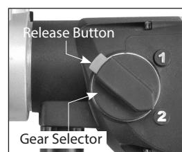
**adjust when the machine is at rest.**
